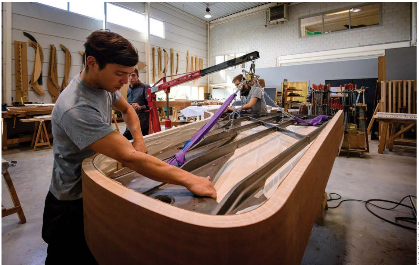
Technicians at Pianos Maene lower the cast-iron frame into a new straight-strung instrument
